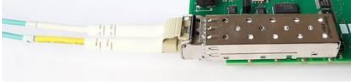
IMAGE 2 - OPTICAL FIBER CONNECTION WITH SFP MODULE
