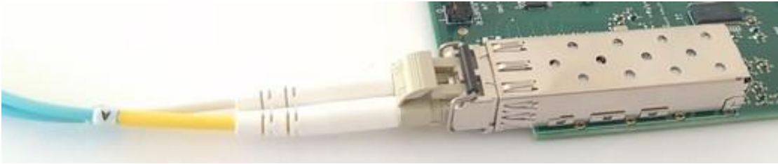
IMAGE 2 - OPTICAL FIBER CONNECTION WITH SFP MODULE
