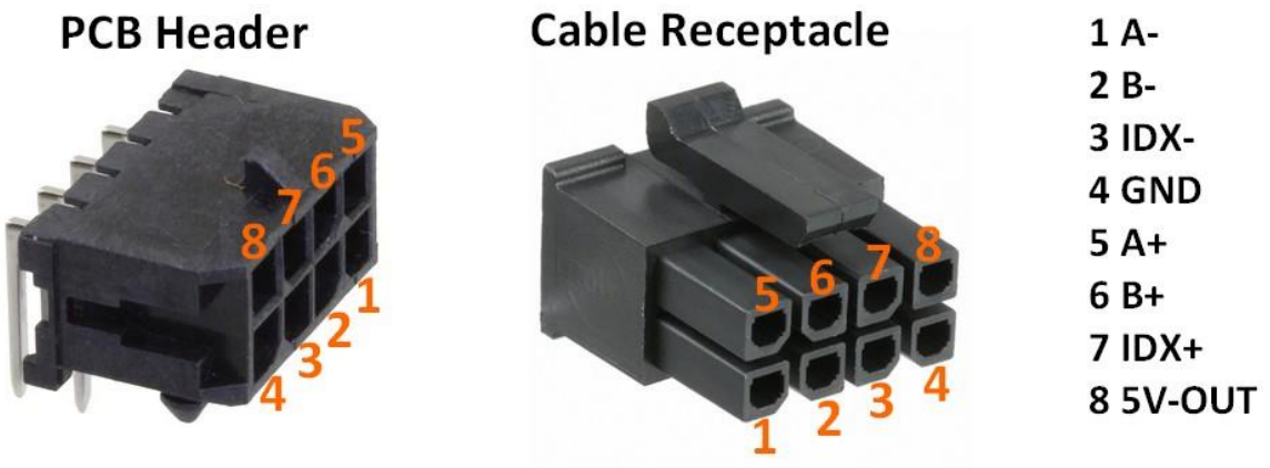
IMAGE 3 – ENCODER CONNECTOR PINOUT
