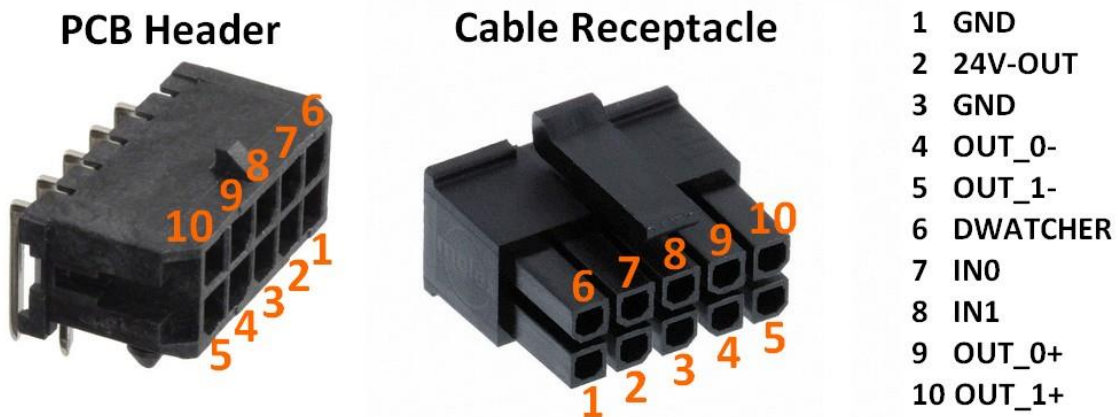
IMAGE 5 – INPUT/OUTPUT CONNECTOR PINOUT
